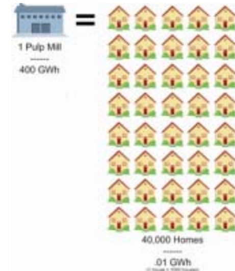
Comparison of the power used by one pulp mill to that of a house.
