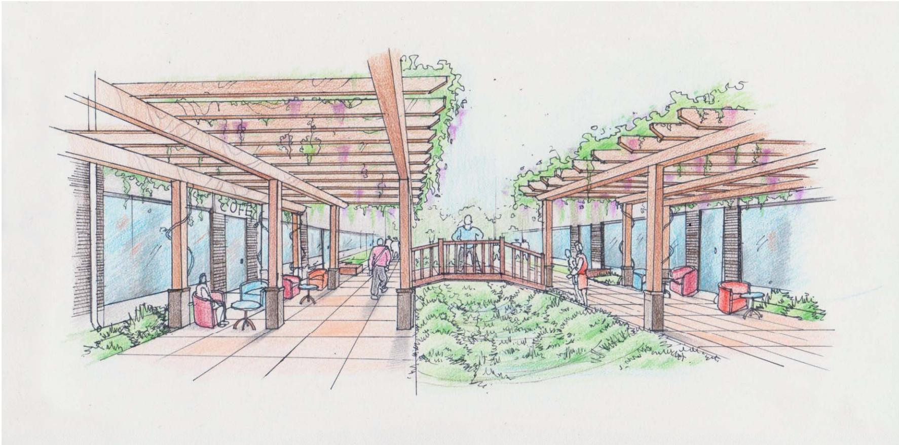
Arbores with creepers irrigated by the rainwater from disconnected downspouts are located on the head of pedestrian paths and eating areas. Wood bridges are cross the pretty landscaping infiltration basin. Midblock pedestrian path is a sweet, peaceful and neat small space for pedestrian to meeting, walking, eating and shopping. Additionally, besides the aesthetic and environmental function, it also provides an education function for public about the sustainable knowledge.
